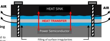
Increasing by means of additional torque during the initial phase change will improve or minimize the material connection, resulting in further improved thermal performance.
